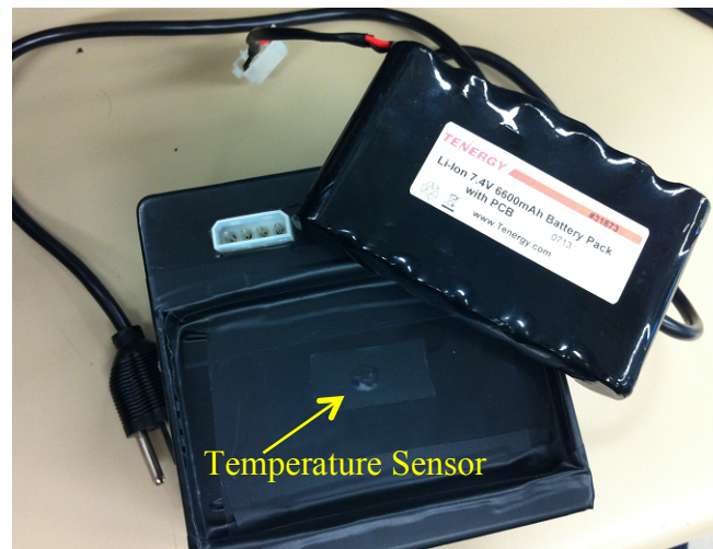
Figure 19: Battery Pack and Charger with Temperature Sensor
