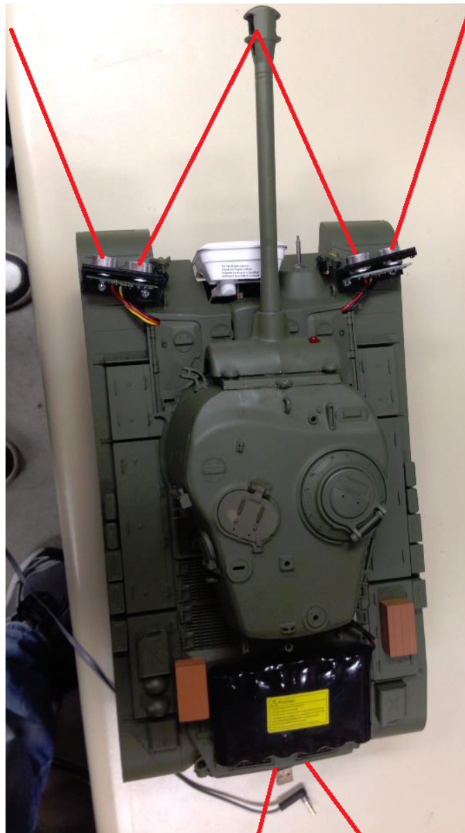
Figure 15: Overhead view of tank and detection angles
